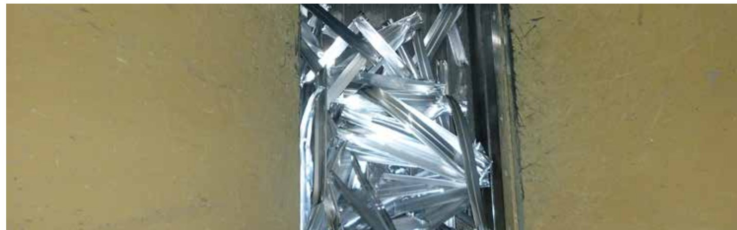
Pressa PM 25 camera pressatura - PM 25 Cabbaging press compacting chamber
